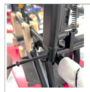
Secure the spacer, bracket and backrest stop bar using the long M6 x 70 bolt.
