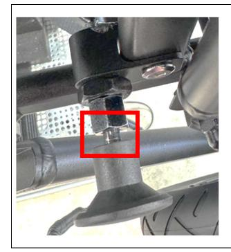
If the toggle handle does not sit flush with the toggle stop, an adjustment will be needed.
