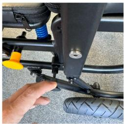
Use the black backrest release toggle to fold the backrest down, then fold the scooter in the usual way.
