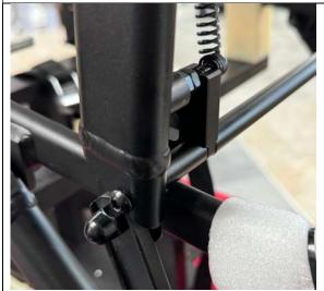
Check all components are secured by moving the back rest forwards and backwards.
