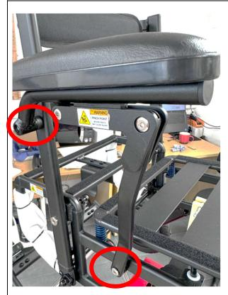
Check the bolts are secured properly without overtightening.
