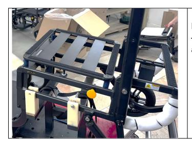
Remove the seat pads from the frame – this will make it easier to fit the armrest kit.
