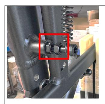
On the left-hand side of the frame, wind in the outer nut to create space for the toggle pin retainer bracket.
