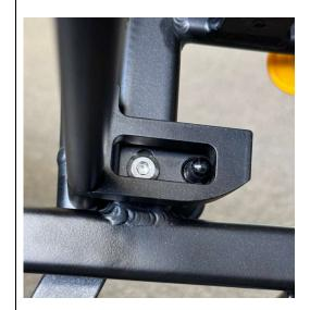
Check the toggle pin sits correctly in the bracket.
