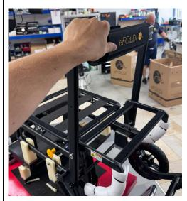
Check the seat back is secure by trying to fold it **without** pulling the backrest release toggle.
