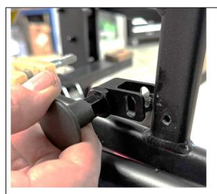
With the backrest in the **DOWN** position, fit the backrest release toggle, per **step III** in the assembly instructions.
