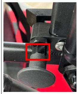
The toggle handle should be flush with the toggle stop, this indicates the pin is fully engaged and the seat back will not move once in the upright position.
