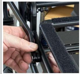
Fit the lower part first to the horizontal part of the frame.
