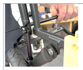
Fix the backrest stop bar and parts indicated in **step V** in the assembly instructions, to the lower part of the backrest frame.
