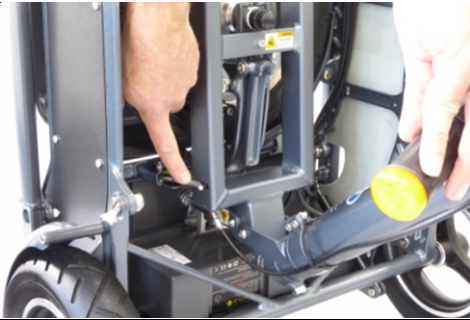
5 While pushing the handlebar down and inwards release the 'E' latch.
