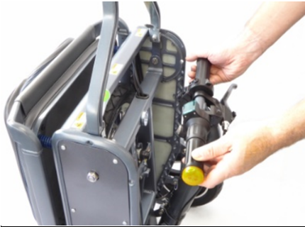
4 Release the handlebar by pulling towards you.
