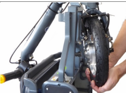
7 Release the front wheel by a sharp pull or twisting.
